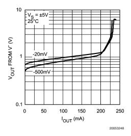
FIGURE 5. V<sub>OUT</sub> vs. I<sub>SINK</sub> (for Various Overdrive)
