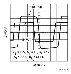
FIGURE 6. Output Overload Recovery
