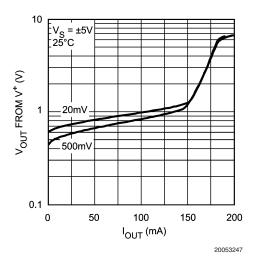
FIGURE 4. V<sub>OUT</sub> vs. I<sub>SOURCE</sub> (for Various Overdrive)
